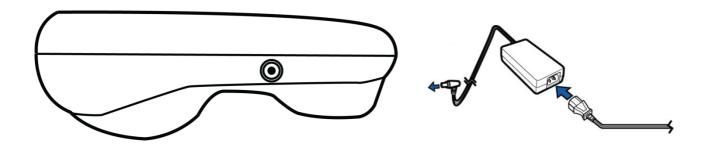
3G terminal: Connect the power cord into the port at the left side of the terminal.
