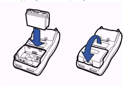
To remove the battery, press the locking tab and pull the battery from its slot.
