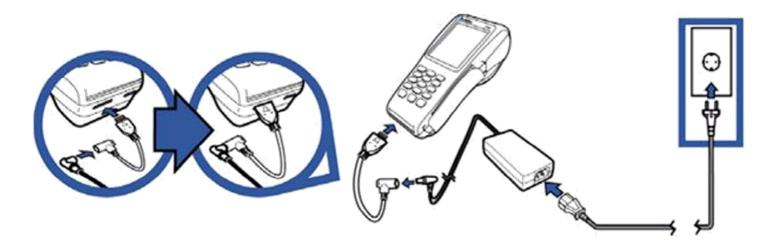
WLAN terminal: Connect the adapter to the main power cord, the power cord to the power supply and the plug to the electrical outlet. The adapter is connected at the bottom of the terminal into the left port.
