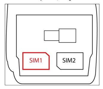
The SIM-card is placed to SIM1-slot beneath the battery so that the chip is facing down and the folded corner points upwards.
